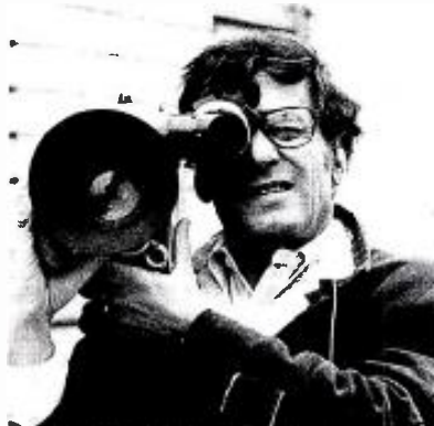
1. First step in KMOX-TV's electronic newsgathering system is portable Ikegami color camera, weighing less than 15 pounds.
